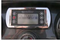
3. Make sure the Wedge is all the way down before you proceed. Make sure you have "down" highlighted in the screen, press "E" once and DONE will change to CAL. Wait 2 seconds and press "E" again and CAL will change back to DONE. The down position is now calibrated.
