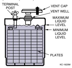
Figure 4-1. Battery Level
