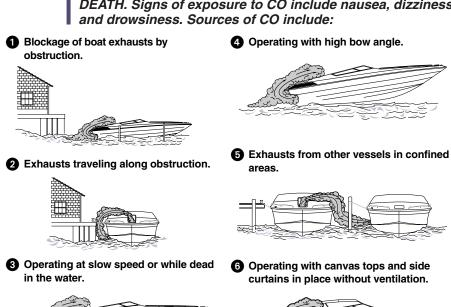
ENSURE ADEQUATE VENTILATION FOR CORRECT AIR MOVEMENT THROUGH BOAT!
