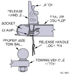
correct ball diameter is marked on the trailer coupler.
