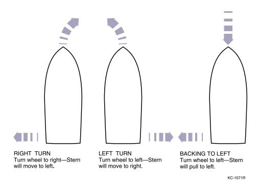
Figure 3-7. Turning With A Rudder
