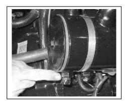
2. Follow the hose from the heat exchanger to the oil/transmission cooler. Remove the hose from the oil/transmission cooler and push the end of the hose low into the bilge to make sure that the hose drains. Remove the drain plug from the oil/transmission cooler and let the cooler drain. Lift the hose that runs from the raw water pump to the oil/transmission cooler so it drains through the cooler. Replace the drain plug in the heat exchanger and in the oil/transmission cooler. Reattach the hoses.
