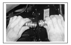
4. On the exhaust outlet end of the exhaust manifolds, there is a hose that runs from the exhaust manifold on the heat exchanger side of the engine to the exhaust manifold on the opposite side. Remove one end of that hose from whichever end is easier to access and push the end of the hose low into the bilge to drain the water from the hose. Reconnect the hose.
