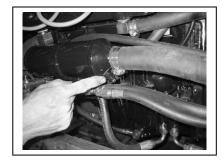
3. Disconnect the hose coupler from the exhaust manifolds. Lower the hose ends into the bilge to make sure that the manifolds drain properly. Reconnect the hose coupler.
