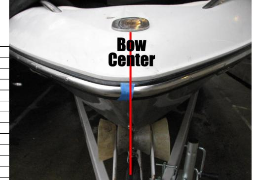
**Step 2 of 8**: Take a piece of masking tape and mark the front (towards bow) of each tower foot at the rub rail to measure off of. Front Post:
