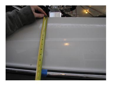
**Step 7 of 8**: At Each Tower Base Measure the Width of the tower base (where the cover will go around at widest point) Front to back and left to right measured in inches
