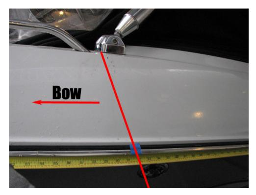
NOTE: If Measured Correct, Port and Starboard sides should be the same
