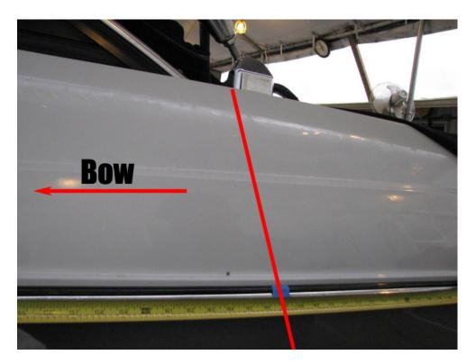
**Step 5 of 8**: Record Starboard Side tower post Measurements in inches from center of the bow to the front of...
