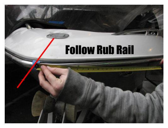
**Step 4 of 8**: Record Port Side tower post Measurements in inches from center of the bow to the front of...
