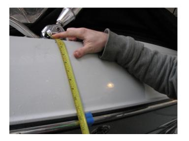
Starboard Rear Tower Post to Center of Rub Rail Measurement
