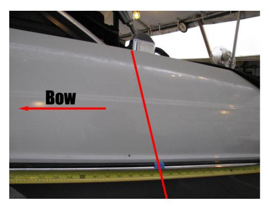
**Step 6 of 8**: At each tower leg base, measure from the center of the rub rail vertically to the start of the tower leg (please follow the contour of the boat)
