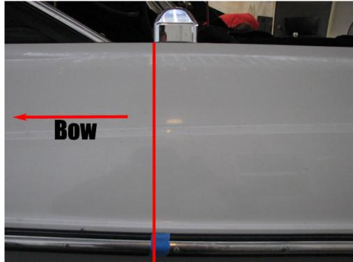
**Step 3 of 8**: Measure from center point of the bow following the rub rail on the Port side (Passenger / Left side of the boat)
