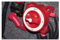
Figure 4-6. Battery Switch
