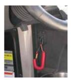
Figure 2-8. Emergency Engine Stop Switch
