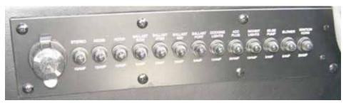
Figure 2-4. Circuit Breaker Panels
